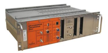
The Trainborne Recorder Unit (TRU) is a New Generation universal Ethernet-based product that records in one unit various train information such as ERTMS signalling data, general signalling data, train diagnostic data, voice or even video information.
